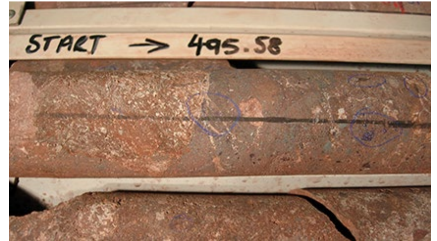
Core sample from the PACE co-funded discovery hole of the Carrapateena deposit, CAR002, showing bornite mineralisation in hematite breccia. (Photo 401840)
