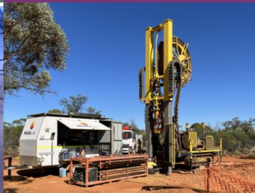
Coil tube drilling rig
