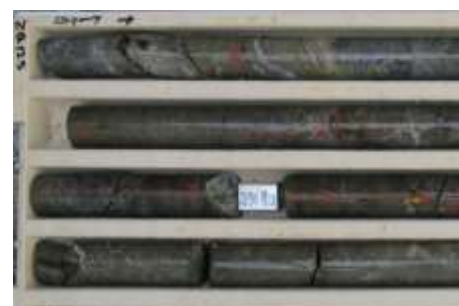
Heemskirk Core: Part of high grade tin zone (7m @ 1.67% Sn average, incl 1m @ 5.55%)
